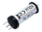
Electromagnetic power reed relay with one contact for closing. It is meant for switching electric circuit of direct and alternating current with frequency up to 10 kHz in communication devices, telemetry, informatics etc.
